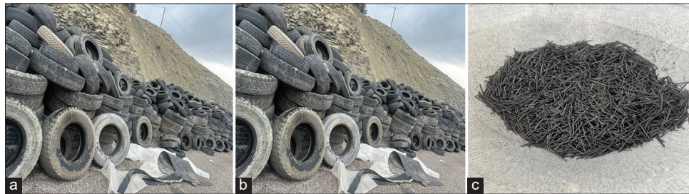
Figure 4: (a) Waste tire (b) steel wire extracted from waste tires. (c) Steel fiber waste tire with 30 cm length
