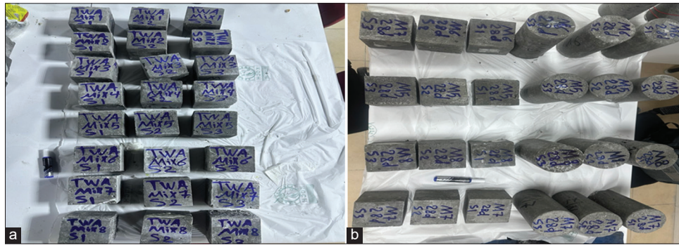
Figure 6: (a) Samples for total water absorption and density test and (b) samples for compressive and splitting tensile strength test
