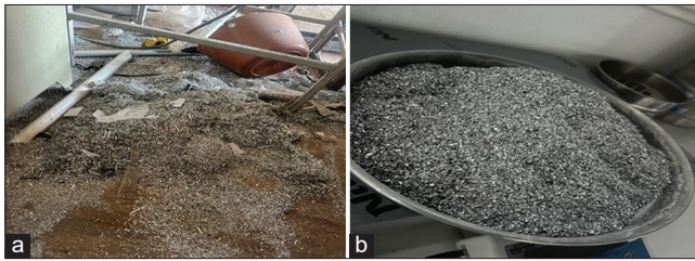
Figure 2: (a) Waste aluminum from factory. (b) prepared waste aluminum for mix
