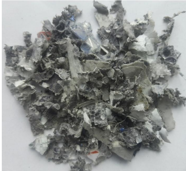
Figure 1: Pieces of silicon sticking to the polymer backsheet. (Taken using a DSLR camera) (Source: by authors)
