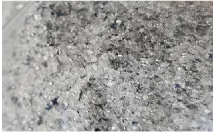
Figure 4: Glass and silicon pieces obtained after the EHF processing (0.1-0.5mm). (Taken using a DSLR camera) (Source: by authors)
