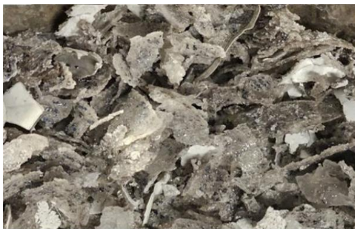
Figure 3: Pieces of polymers obtained after the EHF processing (> 5mm). (Taken using a DSLR camera) (Source: by authors)
