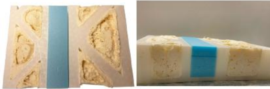
Figure 6: 3D printed mockup of the final wall assembly (scale 1:1). The mockup was created by the study authors using a small-scale 3D printer.
