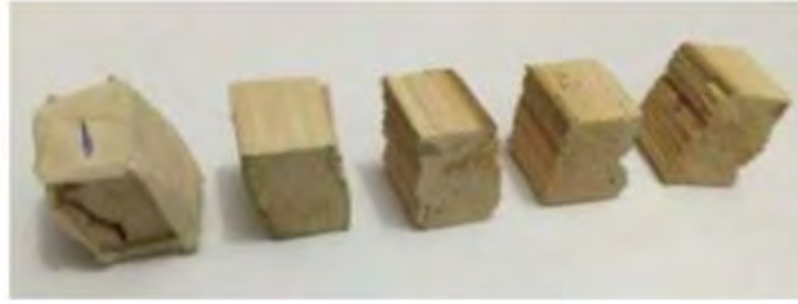
Figure 29. The failure patterns of the compression specimens (Author's own, n.d.)
