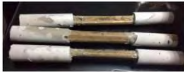
Figure 17. The tension specimens before testing (Author's own, n.d.)
