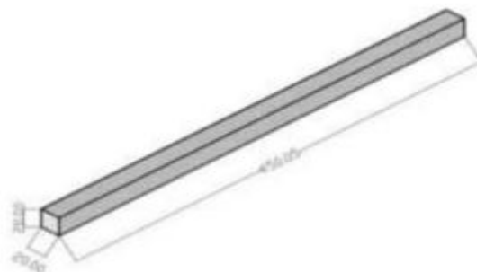
Figure 22. Dimensions of the bending specimen (Author's own, n.d.)
