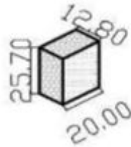
Figure 27. Dimensions of the specimen of compression (Author's own, n.d.)
