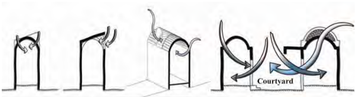
Figure 12. a, b (left and middle): Depicts the new type of crossed vaults. c (right): Depicts the new two-level vaults.
