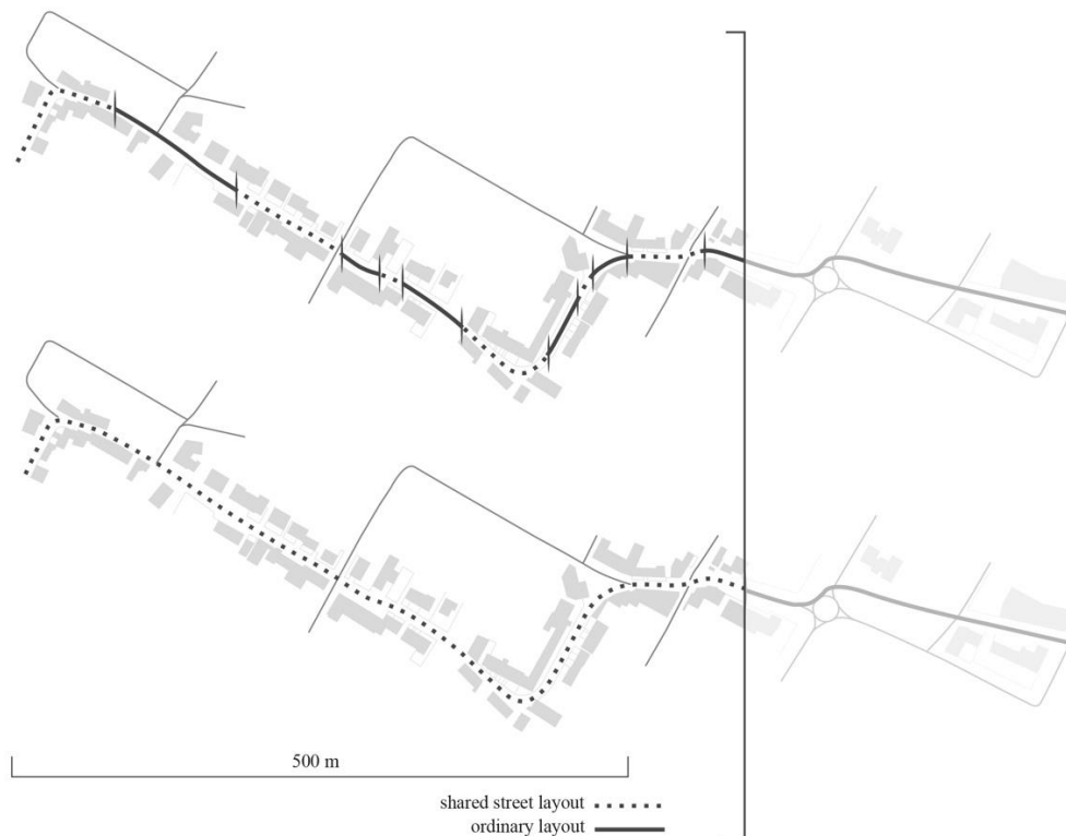
Figure 5. A diagram of the two options of the street partial or total sharing.
