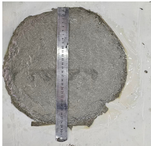
Fig. 3. Slump flow for mix R7.
