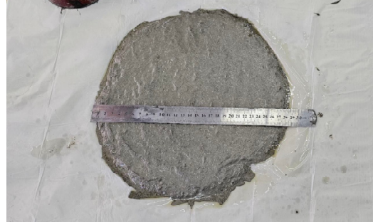
Fig. 2. Slump flow for mix R6.
