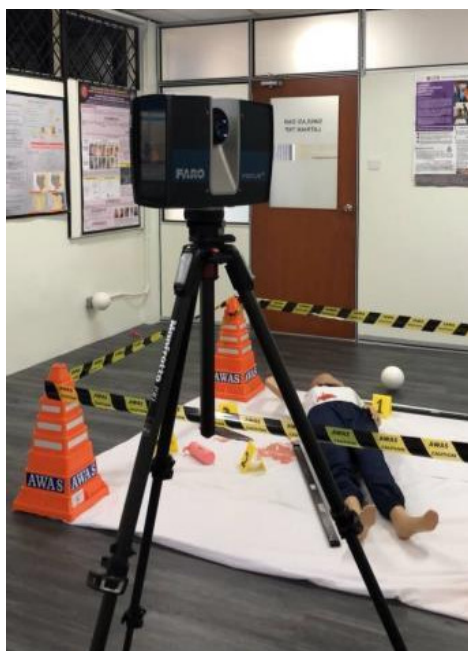
Fig. 3. 3D scanning using Faro Focus laser scanner.
