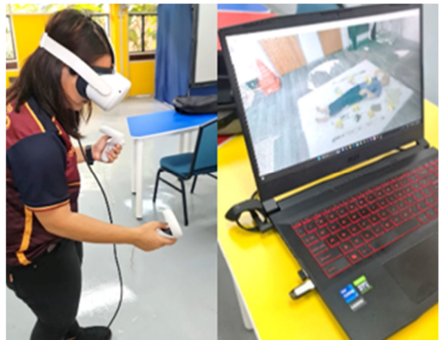
Fig. 4. Importing point cloud into Meta Quest 2 virtual reality.
