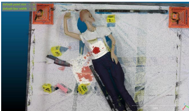
Fig. 5. Point alignment between point-based point cloud (TLS) and texture-based point cloud (CRP).
