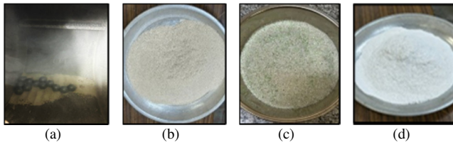
Fig. 1. Process of GP preparation: (a) glass waste, (b) CG, (c) retained on 600 µm sieve, (d) GP.
