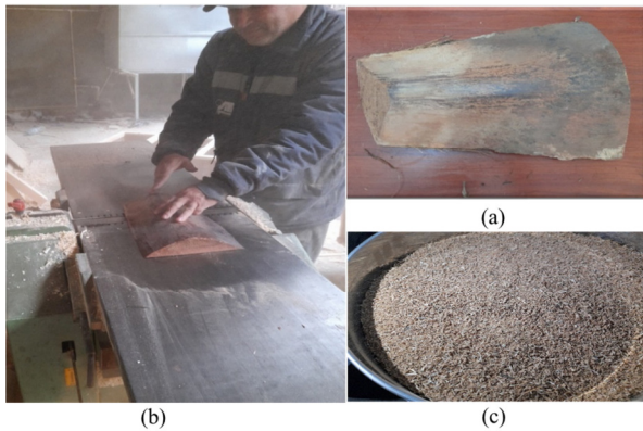
Fig. 3. Processing of DPF: (a) raw petiole, (b) mechanical planing, and (c) final fibers.
