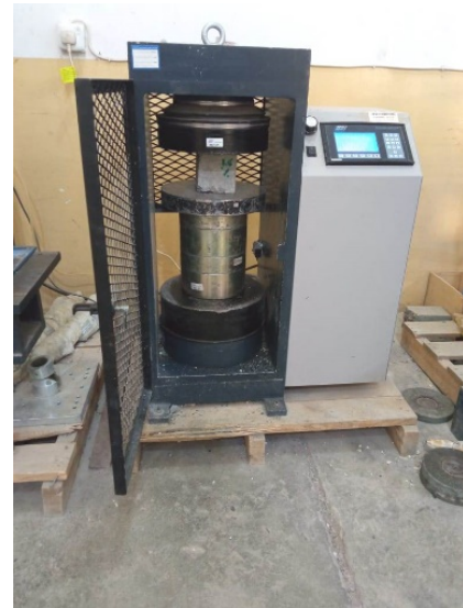
Fig. 2. Specimen under compression test.
