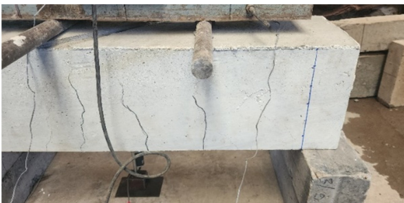
Fig. 12. Crack development in bamboo-reinforced concrete beam (B2) under four-point bending.
