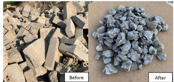
Fig. 1. Concrete waste before and after the crushing process.
