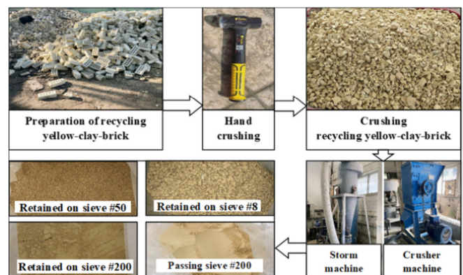
Fig. 3. The process of crushing and grinding waste CB.
