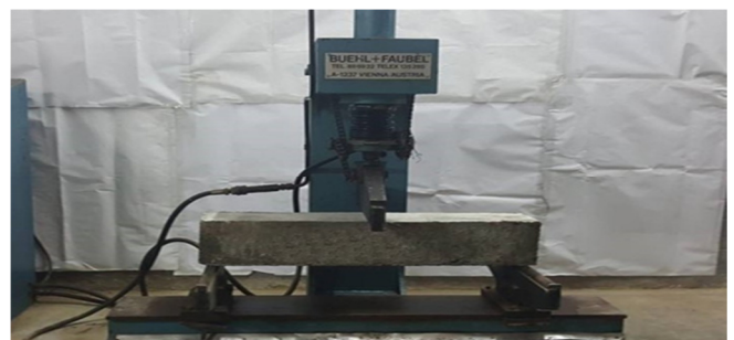
Fig. 4. Flexural strength test.
