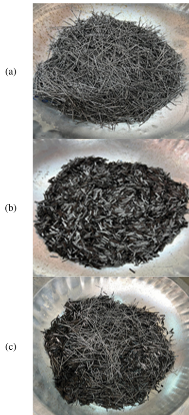
Fig. 2. (a) Steel fiber, (b) carbon fiber, and (c) hybrid fiber (steel and carbon).
