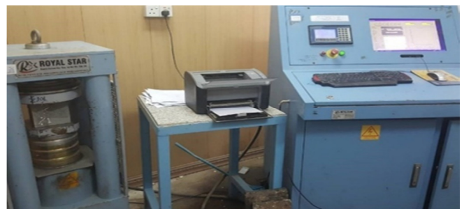
Fig. 3. Compressive strength test setup.
