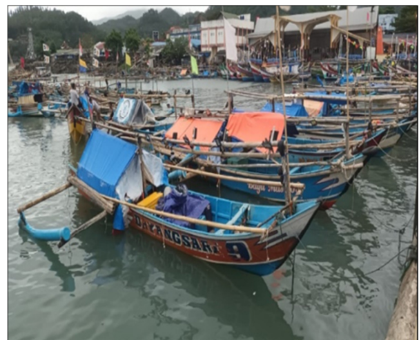
Fig. 1. The float outrigger made of resin on the outrigger boat in Palabuhanratu, Indonesia.
