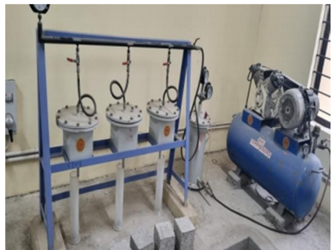
Fig. 2. Concrete permeability test assembly.
