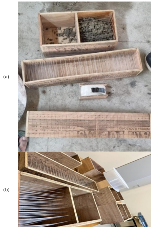
Fig. 1. (a) Formwork using drilled plywood, (b) embedded POF in wood mold.
