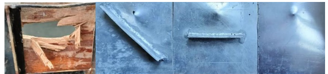
Fig. 7. Experimental deformation of hull configurations after impact.
