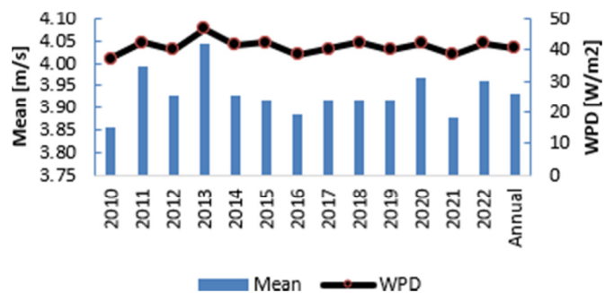
Fig. 6. The annual values of the mean and WPD were calculated using the Weibull parameters.
