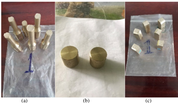
Fig. 14. Mechanical test results: (a) tensile test, (b) hardness test, (c) impact test.
