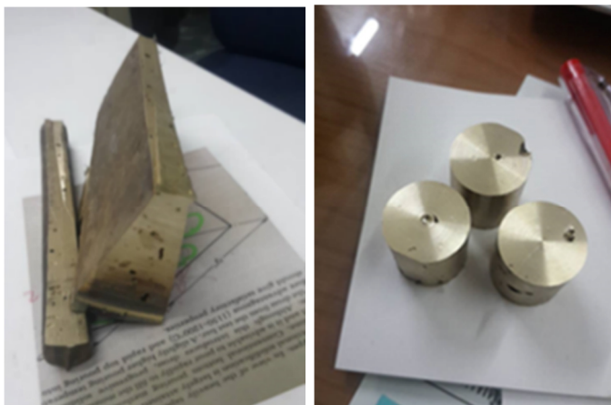
Fig. 2. Damage of the workpiece due to porosity.
