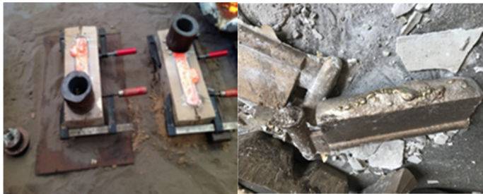
Fig. 1. Inflated upper surface due to gas.
