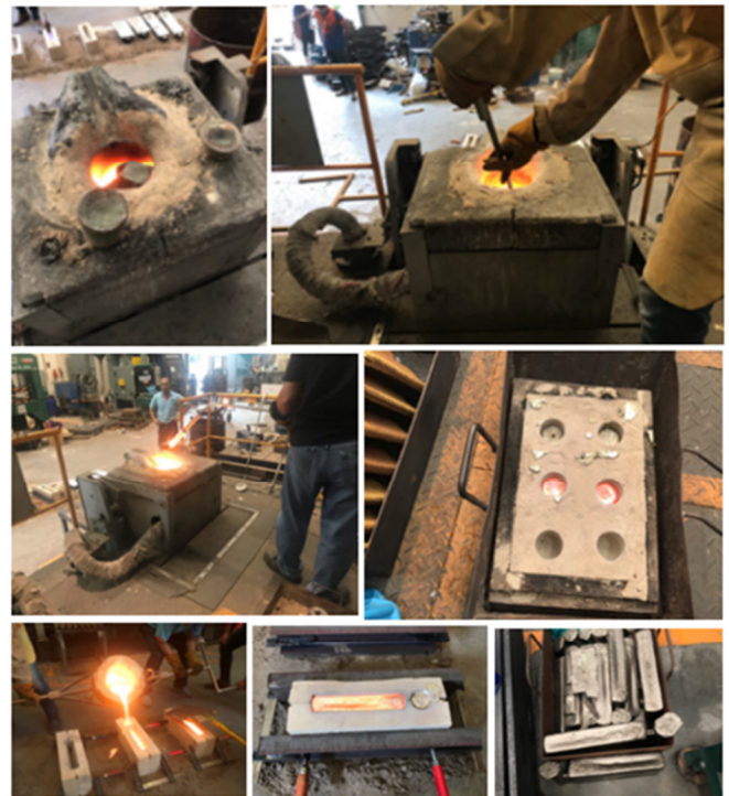
Fig. 6. Casting process of nickel-aluminum bronze.
