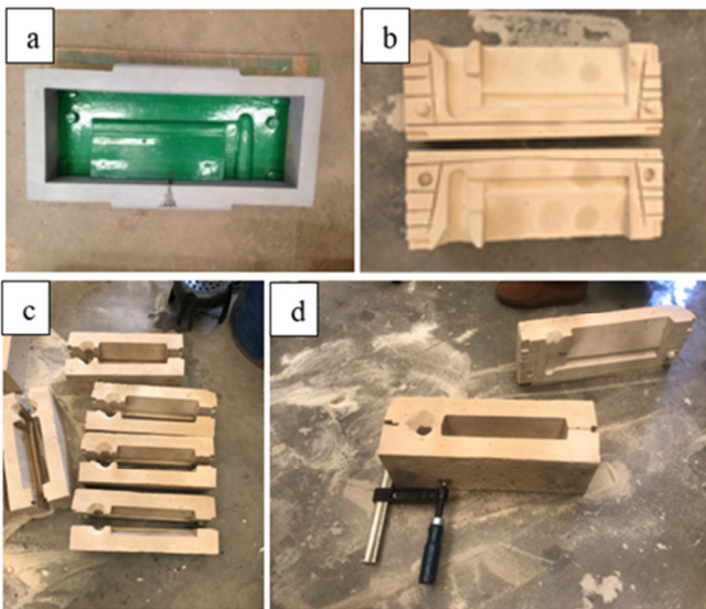
Fig. 4. Experimental assembly: (a) pattern, (b) CO 2 sand casting, (c) vent holes, (d) assembled CO 2 sand casting.
