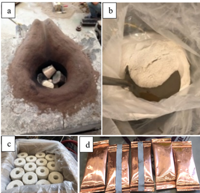
Fig. 5. Materials used for testing: (a) nickel aluminum bronze (AIBC3) scraps, (b) flux compound fluorides, (c) Logas 50 (degassing agent), (d) deoxidizing tube E.
