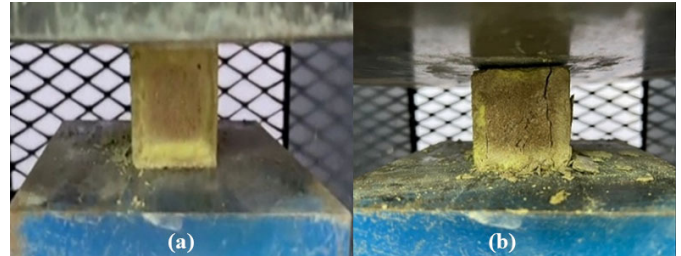
Fig. 6. Unmodified sulfur mortar specimen under compression test (a) and after failure load (b).
