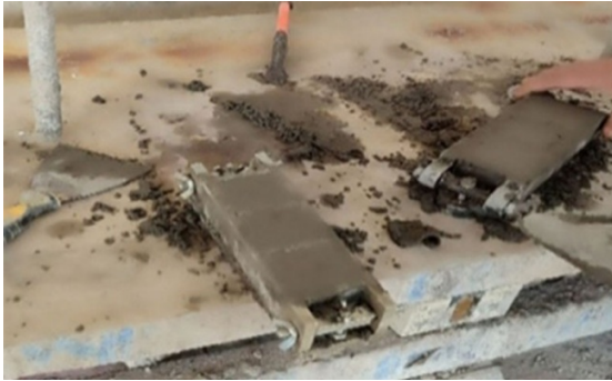
Fig. 3. Cement mortar sample during casting.
