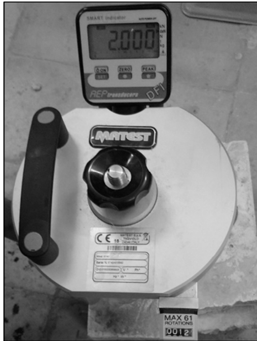
Fig. 4. Equipment used for the direct tensile test.
