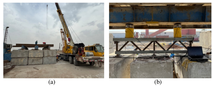
Fig. 12. Loading methodology: (a) system installation, (b) test situation with hydraulic jack over the specimen and all the sensor devices connected to the data logger.
