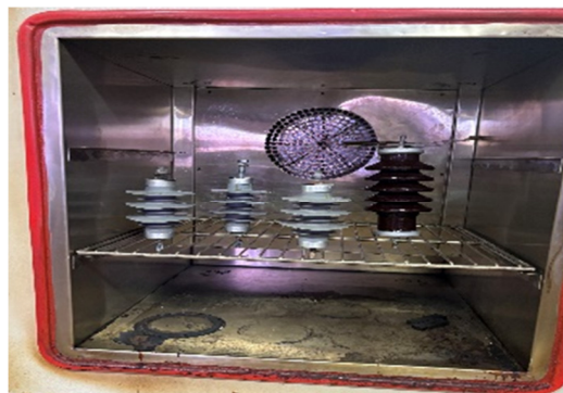
Fig. 6. Experimental setup for temperature ageing at 150°C.
