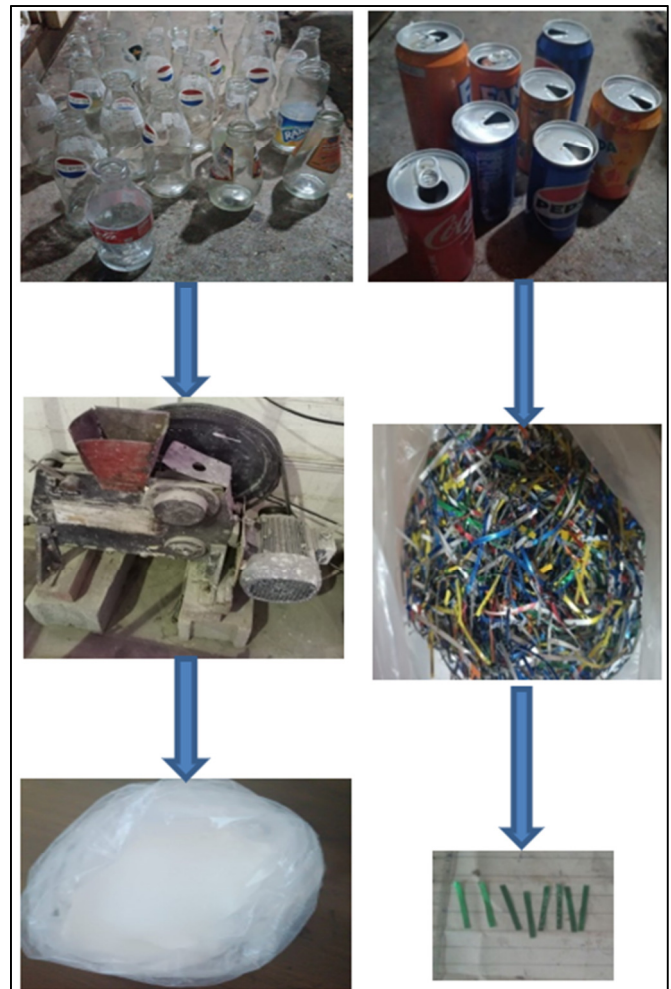
Fig. 1. (a) Glass powder preparation, (b) preparation of aluminum fibers.
