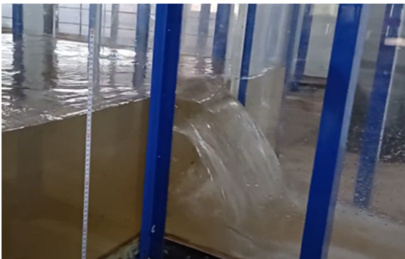
Fig. 5. Overflow condition in the sharp-crested weir without orifice.
