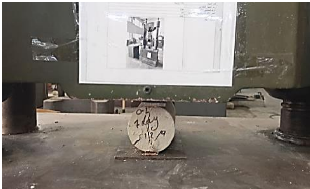
Fig. 4. Cylinder in the splitting tensile strength testing machine.
