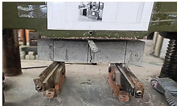
Fig. 3. Prism in the flexural strength testing machine.
