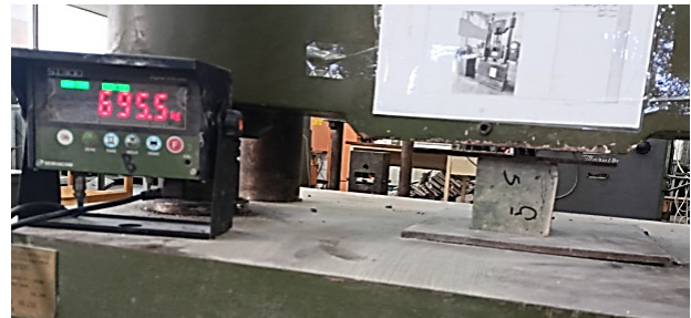
Fig. 2. Cube inside the compressive strength apparatus.
