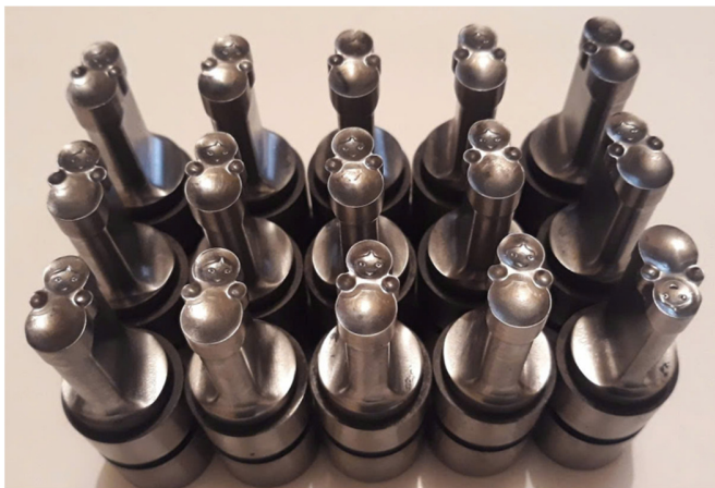
Fig. 4. Tablet punch components with external cylindrical geometry.
