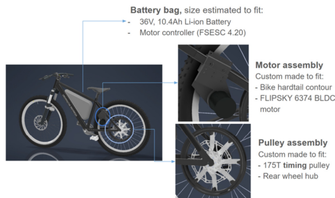
Fig. 3. Placement of the motor assembly and pulley assembly on the bicycle.
