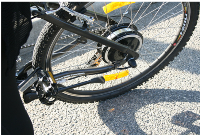
Fig. 1. Typical electric bicycle with a hub-drive design.
