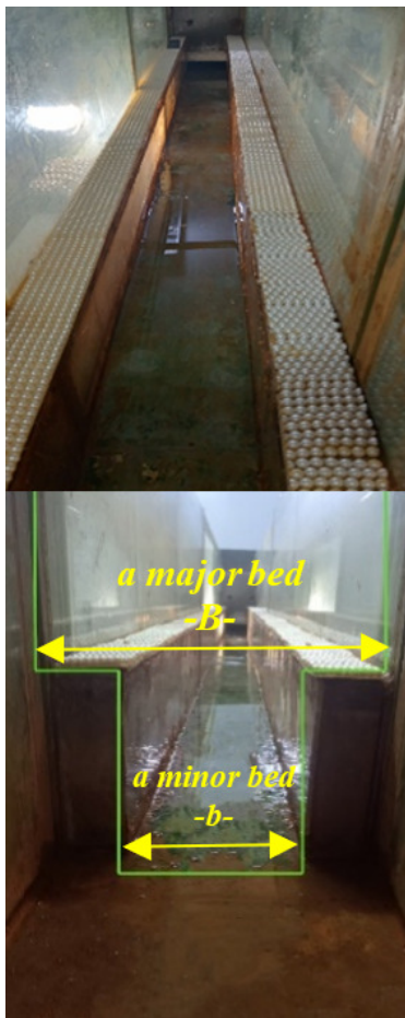
Fig. 3. Composite section channel with rough major bed.
