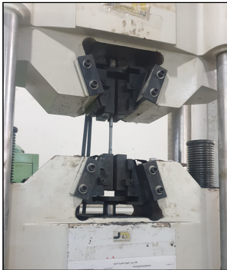
Fig. 12. Testing of steel coupon.
