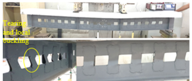
Fig. 26. Mode of failure of specimen BS-E30-T3-L70.
