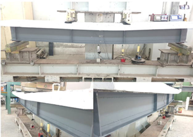
Fig. 23. Mode of failure of specimen BS-E30-T3-L0.
