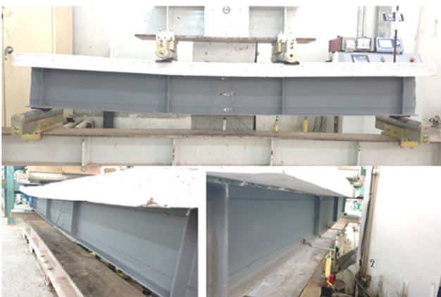
Fig. 24. Mode of failure of specimen BS-E50-T3-L0.
