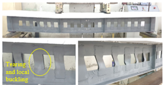
Fig. 27. Mode of failure of specimen BS-E50-T3-L70.
