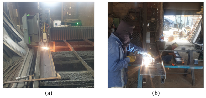
Fig. 13. Fabrication process of specimens: (a) cutting by CNC machine, (b) reconnection by welding plate.
