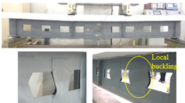
Fig. 30. Mode of failure of specimen BS-E50-T3-L140.
