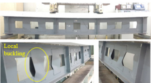
Fig. 31. Mode of failure of specimen BS-E70-T3-L140.
