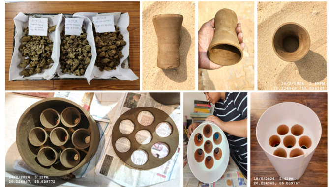
Fig. 2. Soil samples and manufacturing process of earthen Venturi pipe modules and of the earthen indoor air-cooling unit.
