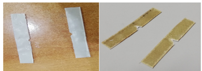
Fig. 7. Notched specimens for the impact test.
