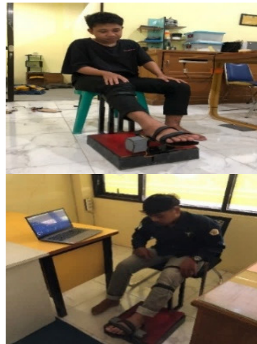
Fig. 9. Experimental setup showing a healthy subject wearing the ankle rehabilitation exoskeleton during testing.
