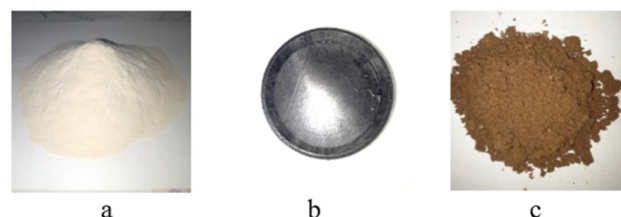
Fig. 2. Materials for mixing: a – biopolymer, b – mixing bowl, c – sand with fine friction.
