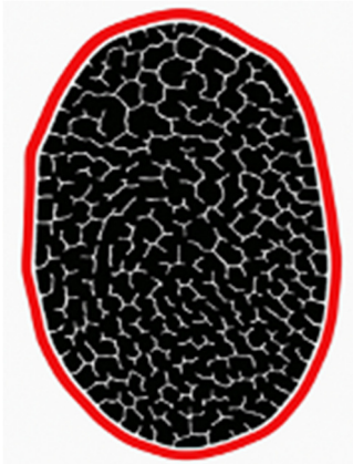
Fig. 3. Fingerprint image after ridge extraction.
