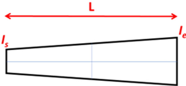
Fig. 2. Longitudinal view of the tapered member at a varying web height.
