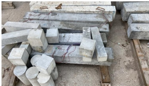
Fig. 5. The samples after mold opening and curing.
