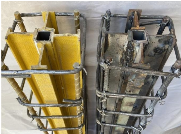
Fig. 2. Reinforcement cage for GFRP and steel I-sections.
