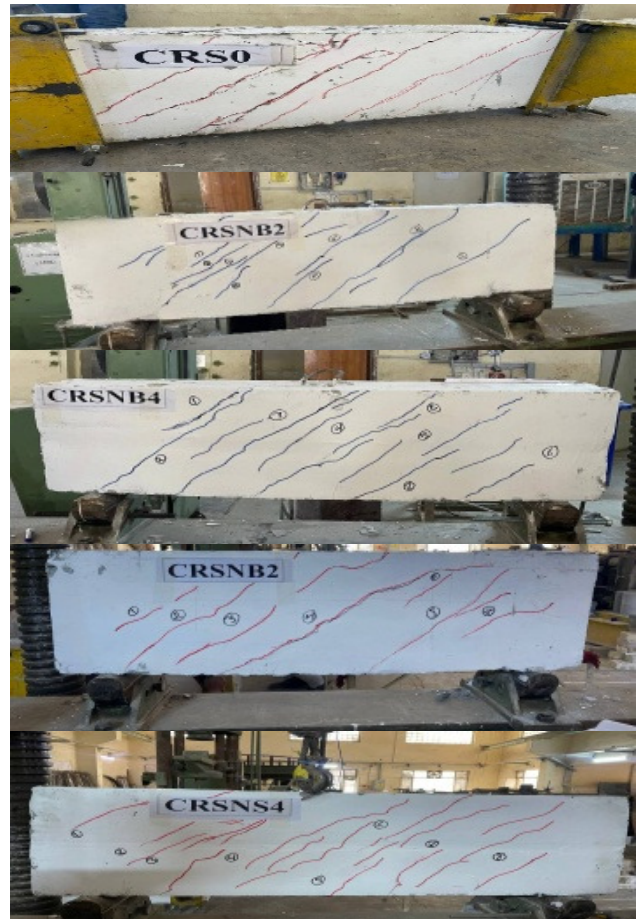
Fig. 4. Failure modes and cracking patterns of the observed deep beam.
