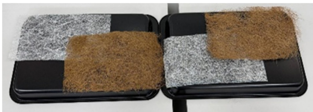
Fig. 2. GF in mat form and prepared DPF (cleaned, dried, and shaped).
