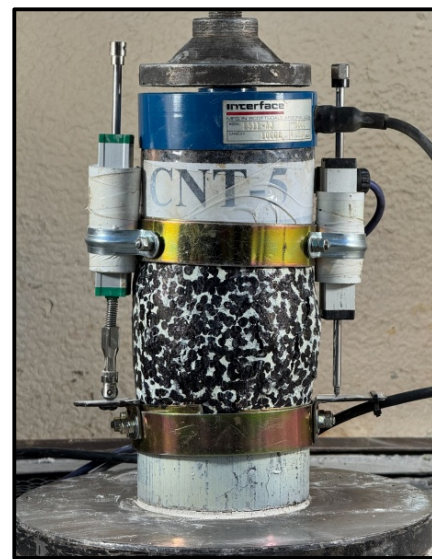
Fig. 3. 8x4 inch asphalt specimen.
