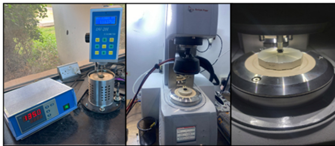
Fig. 4. Rotational viscometer and LAS test using Smart Pave 102e DSR.
