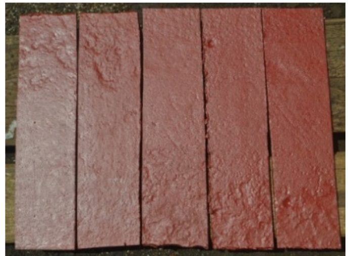
Fig. 4. Epoxy coated ASTM A 36 steel.
