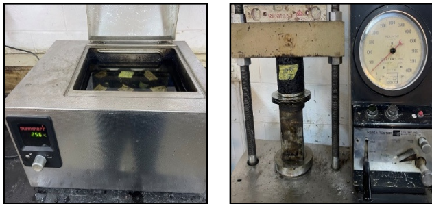
Fig. 6. Compressive strength test.
