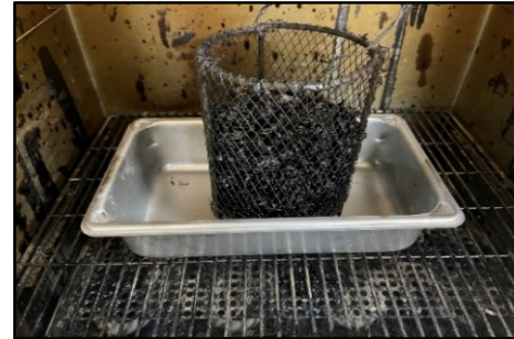
Fig. 4. Drain down test.
