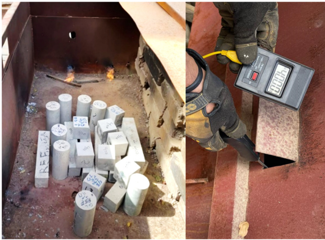
Fig. 3. Fire flame setup used for testing.
