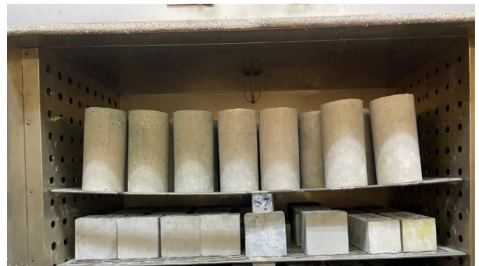
Fig. 2. Placing the sample into laboratory oven.
