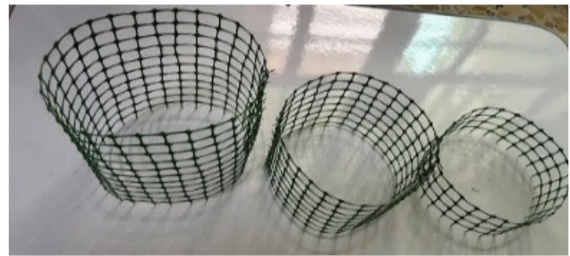
Fig. 1. Loosely skirted cylindrical foundation.
