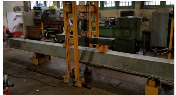
Fig. 11. Bending test of UHPC sheet pile.
