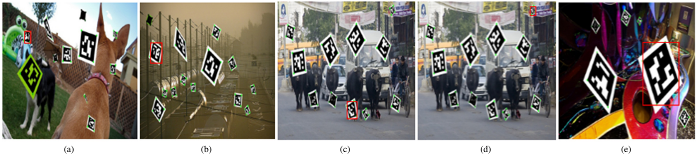
Fig. 3. Examples from the Synthetic-ArUco dataset. Challenging training images are created by superimposing markers of diverse sizes, positions, and spatial placements onto background images sourced from the COCO dataset. Selected instances from the detection dataset: (a-e) correspond to classes 1-5.
