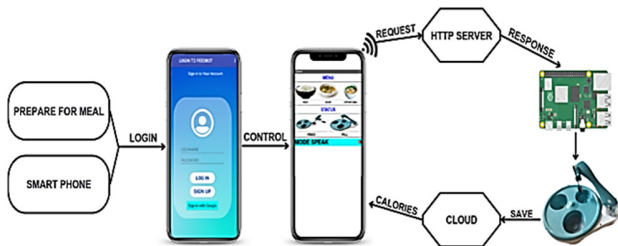
Fig. 5. Structure of the control and communication system of CareFeeder.
