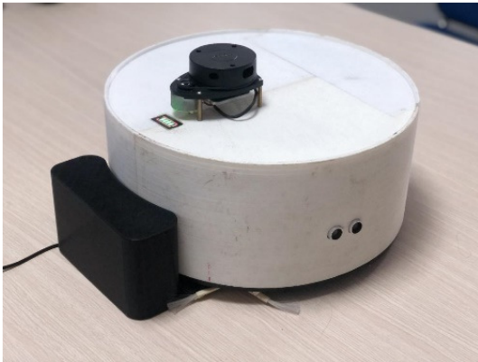
Fig. 9. Realistic model of the automatic vacuum-cleaning robot.
